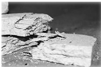
Asbestos insulation board (AIB)
